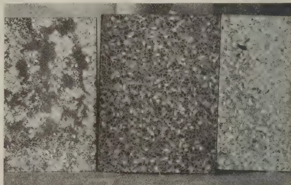
CONCRETE SLABS FOR DECORATIVE WORK. THESE ARE COMPOSED OF CEMENT AND FLORIDA BEACH SAND CONTAINING SHELLS, THE TOPPING BEING A 1:2 MIX, AND HIGHLY POLISHED
